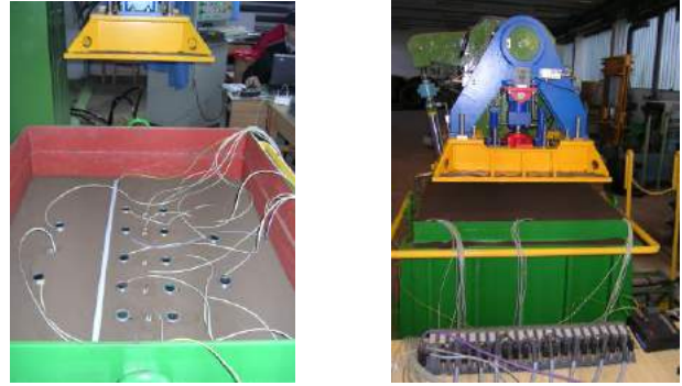
Fig. 9. The installation of the sensors
