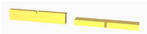
Fig. 1. Vertical (left) and horizontal (right) orientation of test specimens in the tray of additive manufacturing system
