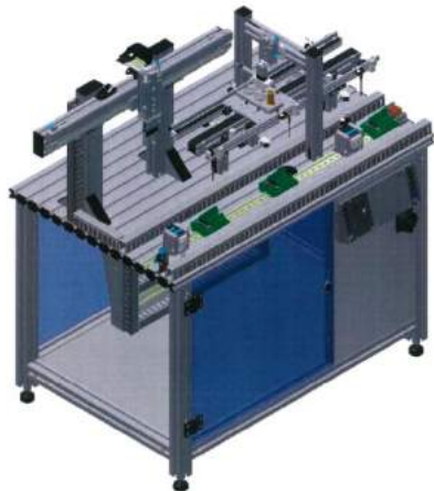
Fig. 3. Quality Handling station (Festo didactic, 2013)
