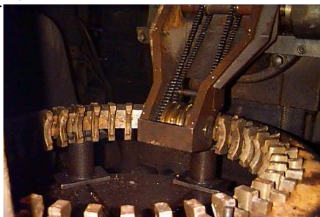
Figure 16. Helical worm – internal teeth worm wheel drive
